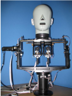
Binaural & binocular heads mounted onto a pan-tilt device
