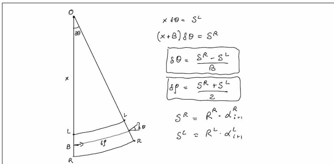
Screen 2: Shift and rotation in a differential drive in terms of the rotations of the two wheels
