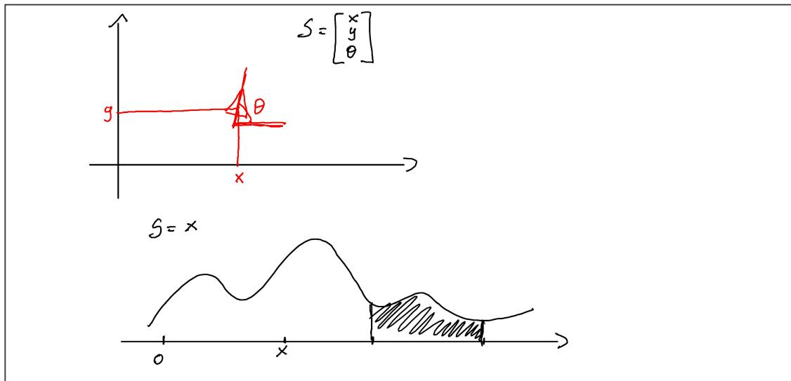
Screen 1: Robot configuration for a wheeled robot (up) and the probability distribution in the case of a robot moving in a 1D space
