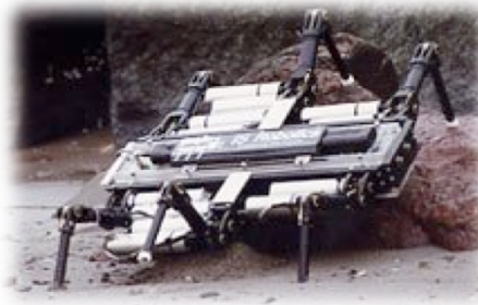
Autonomous legged robot (Tactile & Vision sensing)
